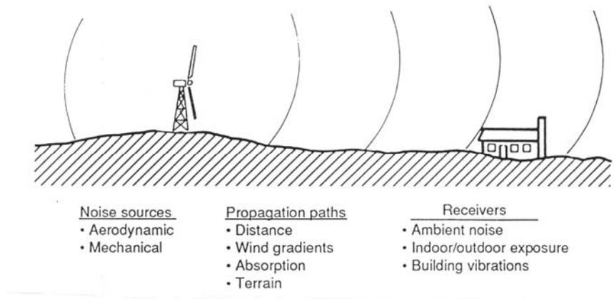
Figure 1: Examples of sources, receivers, and propagation paths
