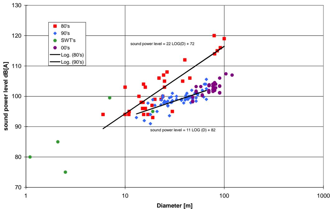
Figure 13: Sample wind turbine measured sound power levels
