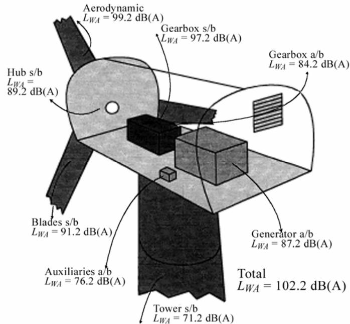
Figure 6: Components and Total Sound Power Level of a Wind Turbine, showing structure-borne (s/b) and airborne (a/b) transmission paths [Wagner, 1996].
