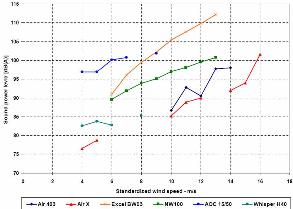
Figure 10: Summary of NREL study of small wind turbine sound: sound pressure level vs. wind speed, with the sound recorded downwind from the turbine [Migliore, 2003]
