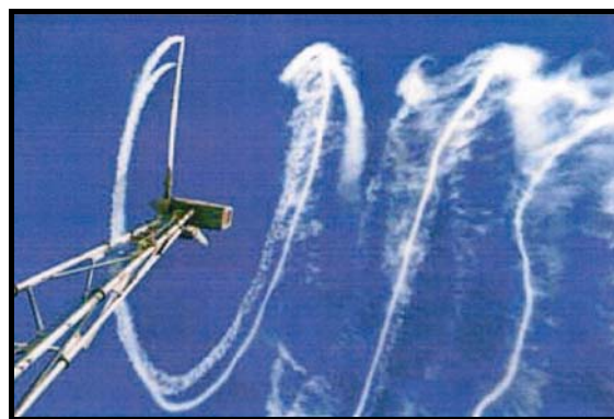
Figure 5 A trace from one blade of a wind turbine
