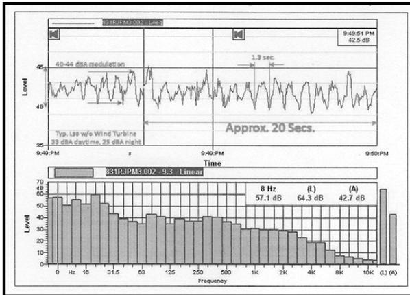
This figure is taken from work done by Richard James in Wisconsin [James 2008] and shows in the top half of the figure, for a single wind turbine, the A-frequency weighted sound level rising and falling in synchronization with the rotation of the blades. The lower half gives a 1/3 octave band analysis of the sound at the point in time shown by the vertical line in the centre of the time history.
