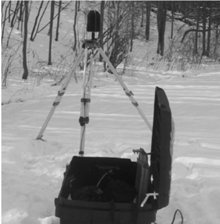
Fig 1: Hayes McKenzie (Ecogen) Typical Background Sound Measurement Setup
