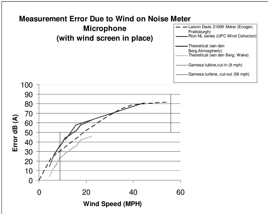
**Fig 3: Noise Meter Microphone Error (Bolton)**
