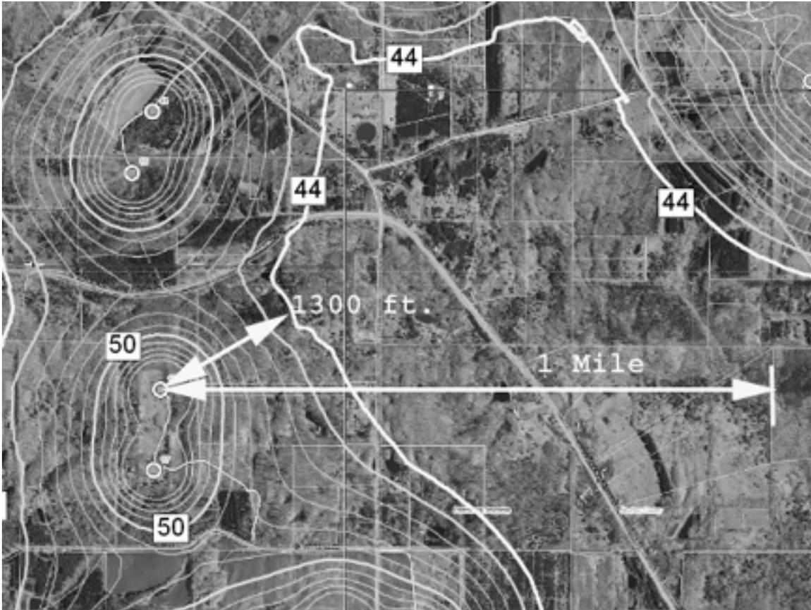
Fig 7: Excerpt of Expected Sound Contours of WindFarm Prattsburgh Turbines, with Distance Scales
