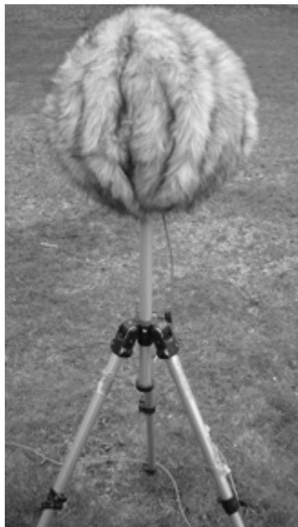
Fig. 8: Secondary Noise Shield from Delta Co., Denmark
