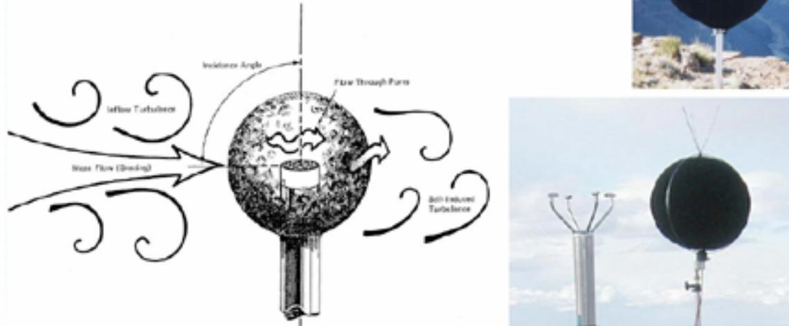
Fig. 7: Wind Screen for Limiting Wind-Induced Microphone Noise
