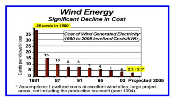
In the early 1980's, when the first utility-scale wind turbines were installed, wind-generated electricity cost as much as 55 cents (C\$) per kilowatt hour. Now, state-of-the-art wind power plants at high value wind sites are generating electricity at costs as low as 6 cents/kWh (C\$), a price that is competitive with many conventional energy technologies. Costs are continuing to decline as more and larger plants are built and advanced technology is introduced.
