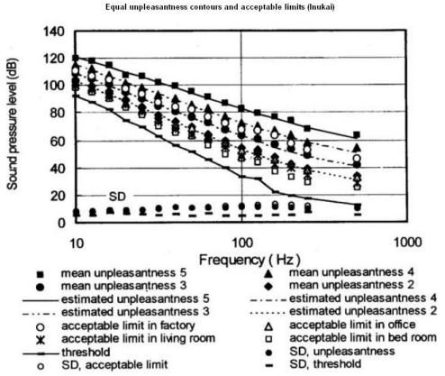
The numbers 1, 2, 3, 4, 5 refer to the unpleasantness level. All levels of unpleasantness are approximately linear with a negative slope of 5 - 6dB per octave. The acceptable limits for different locations are all above the hearing threshold in this laboratory setting. For example, the self-adjusted acceptable limit in an assumed bedroom is more than 10dB above threshold, but this might not be replicated for long term exposure at night in a real bedroom.
