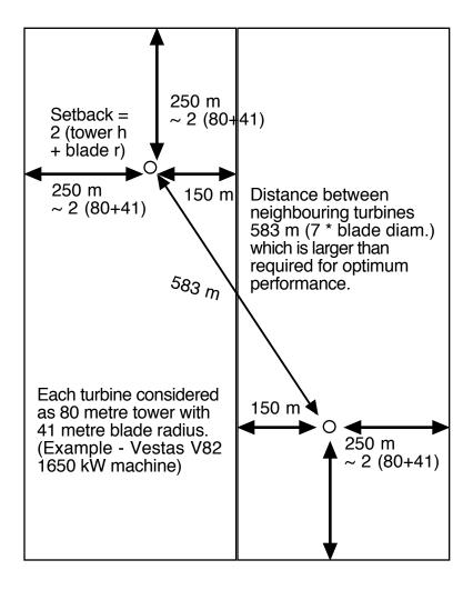
This figure shows that a 2 times tower height plus blade radius could be applied for the 80 metre towers currently being considered, and would not restrict farmers who wanted to work together to develop the wind resource.
