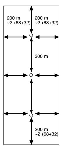
Each turbine considered as 68 metre tower with 32 metre blade radius. Example - 1000 kW machine. Up to three turbines could be installed on 100 acres with distance between neighbouring turbines of 300 m ( 4.7 \* blade diam) which is larger than required.
