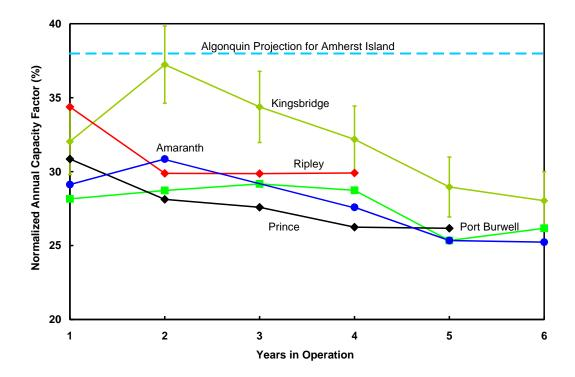
operating for 4 years or more, these normalized capacity factors are shown as a function of the number of years of operation in the figure above. The uncertainty (standard deviation) in the values of  $(v/v_0)^3$  is reflected in the uncertainty in the normalized annual capacity factor. This is demonstrated in the figure only for the Kingsbridge data set.
