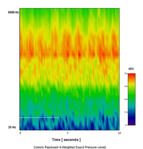
Figure 1: Spectrogram of Sound Pressure Levels Measured near a Vestas 1.8 MW Wind Turbine Generator.
